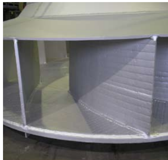
Impeller protected by resurface welding.
