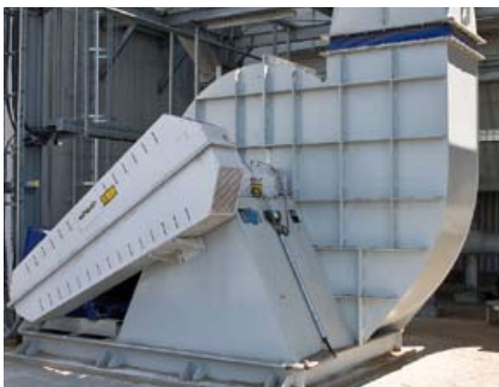
Transport fan with belt drive
