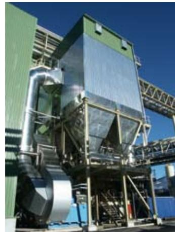
Chamber filter for cleaning flue gas
