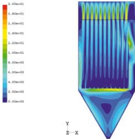
These flow simulations show that velocities in the entire crude gas area are approximately equal and that there is consequently a homogenous distribution of particles.
