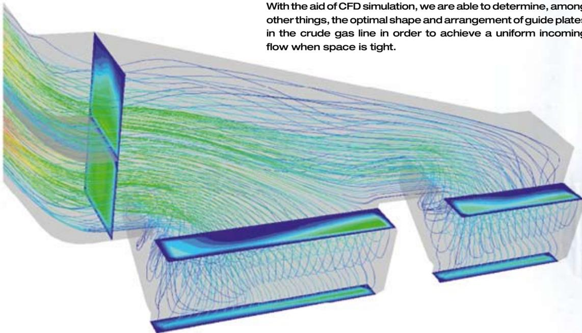
With the aid of CFD simulation, we are able to determine, among other things, the optimal shape and arrangement of guide plates in the crude gas line in order to achieve a uniform incoming flow when space is tight.
