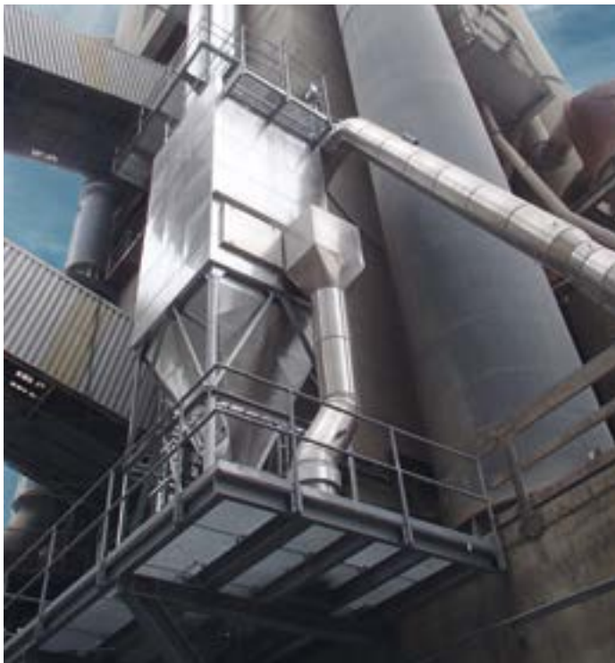
The Xmercury split preheater system implemented at W&P Zement's production facility in Wietersdorf, Austria.
