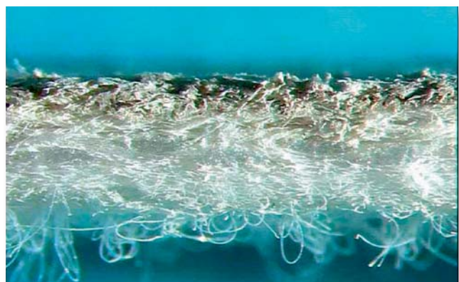
Figure 11: Cross-section of polyester needle felt after a service life of 66 months
